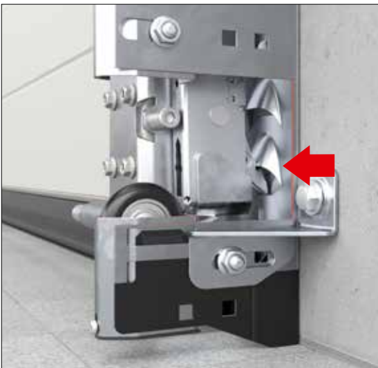
The locking hook of the anti-lift kit automatically latches if the door is forced upwards.
