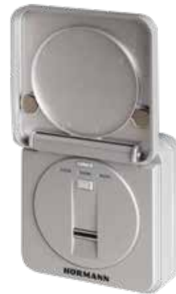
Radio finger-scan FFL 25 BS For 2 functions and up to 25 fingerprints with hinged cover, recessed and surface-mounted fitting possible, plastic housing painted in White aluminium RAL 9006
