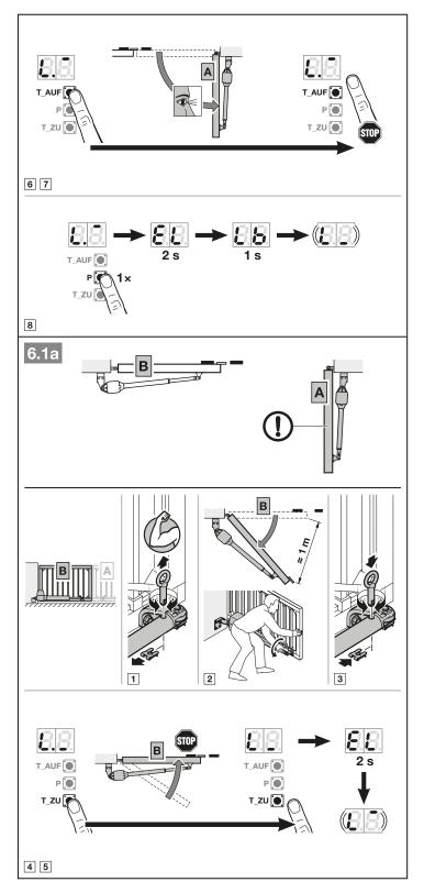
If the position taught in by the limit switch is not the desired end position:
