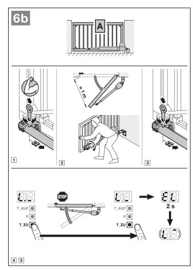
If the position taught in by the limit switch is not the desired end position:
