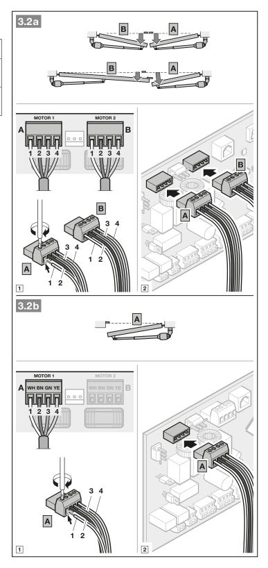
In the operator, plug the connection cable into the socket on the motor connection circuit board.
