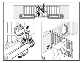
During a power failure, you have to open and close the gate system manually. For this, you have to disengage the operator.
